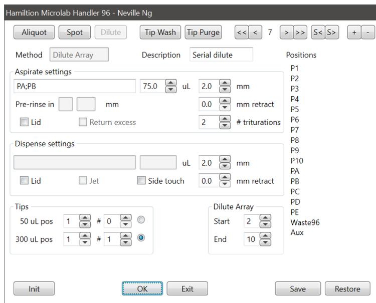
Figure 3. Serial dilution program interface
