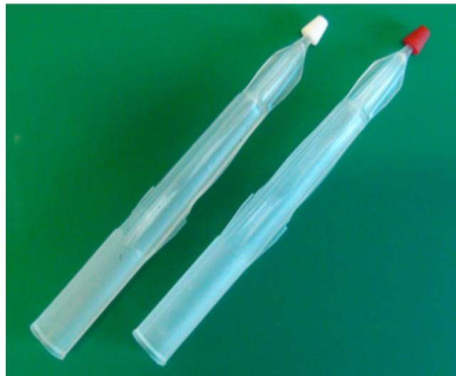
**Figure 1.** MITRA® device. The volumetric absorptive matrix sampling sampler consists of a hydrophilic polymeric tip, which absorbs an accurate sample volume (about 10  $\mu\text{l}$ ) within 2-4 s by wicking, attached to a molded plastic handle. The white-tipped sampler is unused while the red-tipped sampler contains a sample of dried blood. (Reprinted with permission from [14]. Copyright 2014. American Chemical Society).
