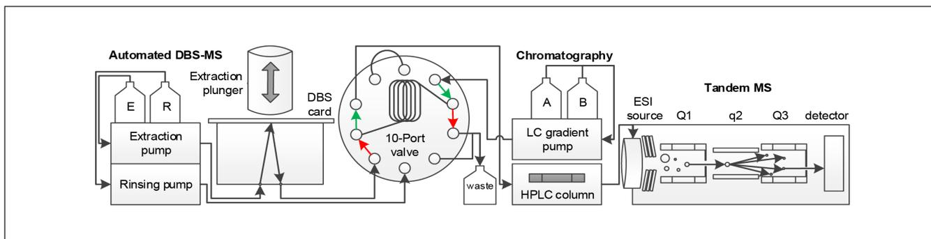
**Figure 4.** Flow scheme of the automated DBS-LC-MS/MS approach.
