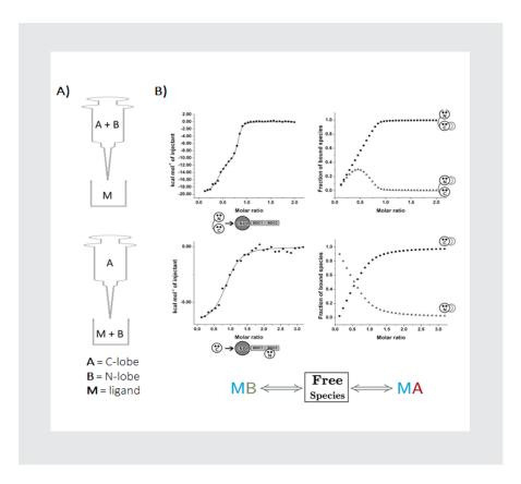
**Figure 2**. A) Schematic representations based on the AFFINImeter MAB code, of the ITC titration of CaM into CNBhD-BDC1-BDC2 (up) and the titration of C-lobe into a mixture of CNBhD-BDC1-BDC2 and N-lobe (down). B) Fitted isotherms of the two titrations (left) and species distribution plots (right). The AFFINImeter competitive model used is shown at the bottom of the figure. Adapted with permission from figure 7 of [19], published by Cell press.
