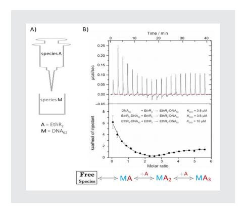
**Figure 1**. A) Schematic representation of the ITC titration of EthR into DNA62 based on the MAB code of AFFINImeter where "A" is the EthR dimer (in the syringe) and "M" is DNA62 (in the calorimetric cell). B) ITC data for the titration showing the thermogram (upper panel) and the fitted isotherm (lower panel). The AFFINImeter tailored model used is shown at the bottom of the figure. Adapted with permission from figure S12 of [18], published by The Royal Society of Chemistry.
