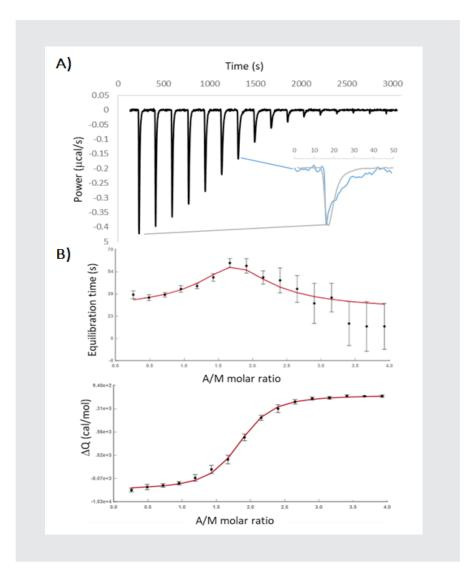
**Figure 6**. ITC data of a 1:1 binding interaction used for thermodynamic and kinetic analysis. A) Thermogram and overlaid of two peaks from the beginning and mid-titration to highlight the peak broadening observed at mid-titration. B) Equilibration time curve (up) and binding isotherm (down) obtained from the thermogram. These two curves are globally fitted in KinITC-ETC to retrieve thermodynamic and kinetic information.
