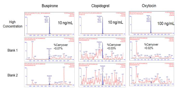
Figure 3. Chromatograms from the carryover study of the three compounds. The top chromatograms for each compound are from sample injection, followed immediately by blank injections reflected in the middle and lower chromatograms. Compound-specific gradient conditions were used.
