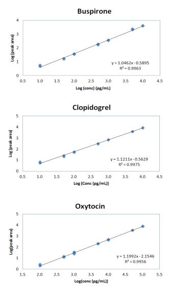
**Figure 5**. Plot of peak area versus concentration for a serially diluted solution of test compounds in human plasma. Each concentration was injected in triplicate and plotted. A compound-specific gradient and scan rate of 0.1 s were used.
