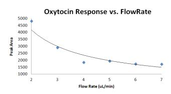
Figure 7. Plot of MS peak area versus flow rate showing response increase with decreasing flow rate from 7  $\mu$ L/min to 2  $\mu$ L/min.
