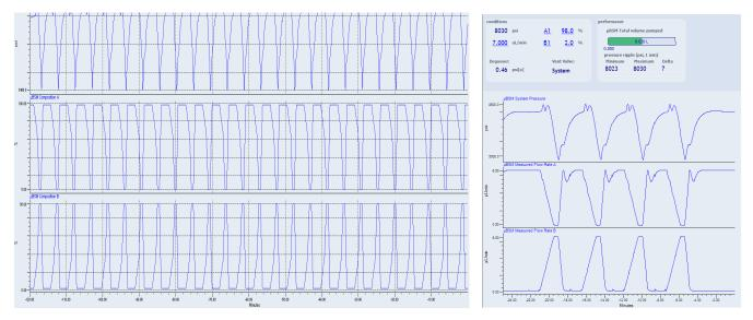
**Figure 2.** A screen capture of the ACQUITY UPLC M-Class Binary Solvent Manager showing system pressure change during sample analysis. On the left is the pressure history using the HSS T3 iKey in a two hour period, and on the right the system pressure using the BEH iKey for four sequential injections. In each graph, the top trace is the system pressure, and the middle and bottom traces are composition changes in channel A or B, respectively.
