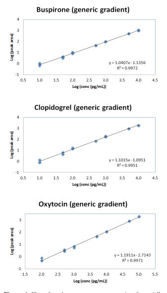
Figure 6. Plot of peak area versus concentration for serially diluted solutions of test compounds in human plasma. Each concentration was injected in triplicate and plotted. Generic gradient conditions and a scan rate of 0.036 s were used for all compounds.
