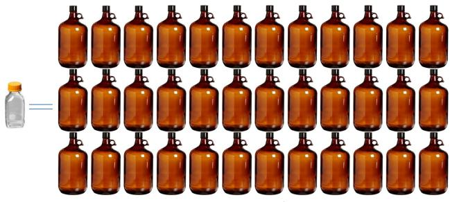
**Figure 9**. Comparison of relative solvent consumption of ionKey running at 7  $\mu$ L/min flow rate vs. analytical scale chromatography running at 1 mL/min flow rate is displayed. The figure shows that consuming 1 L solvent on the ionKey/MS System running continuously at 7  $\mu$ L/min for 99 days or 35,700 injections at 4 min run time, is equivalent to thirty six 1-gallon bottles using an analytical scale system.
