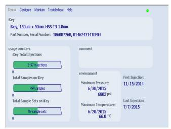
**Figure 8**. Screen capture of the HSS T3 iKey history, showing the number of injections (2197) and maximum operating pressure.
